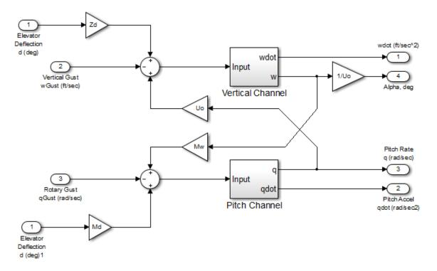
**3** Specify uncertain variables for the gain blocks Zd and Mw in the Aircraft Dynamics Model subsystem.
