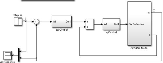
**2** Define a margin analysis point at the output of the Airframe Model block.
